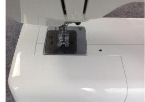
Select Straight Stitch on the Selector dial, the stitch Length doesn't matter because the darning plate is fitted, and the fabric will not feed through the machine.
